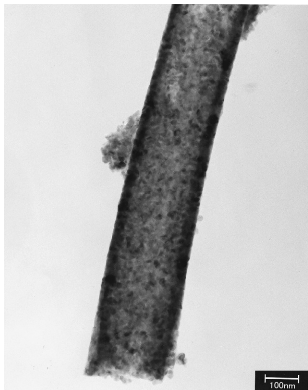
Fig. 5. TEM image of the rectangular column-structured titanium oxide crystals.
